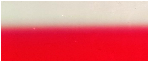
Unclear transition between white and red because of incorrectly installed bulb.
