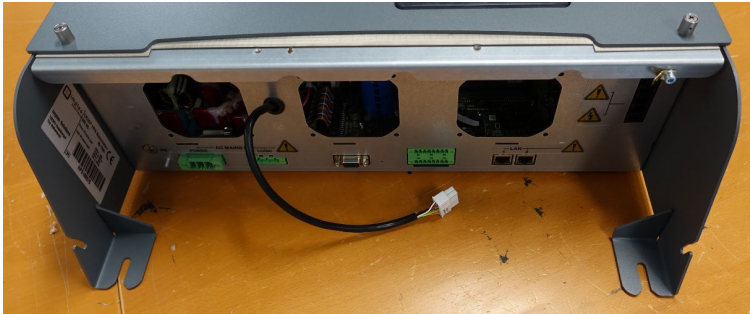
Bottom view of a CEDD HPS Basestation without fan bracket installed. The black cable was connected to the fan bracket.
