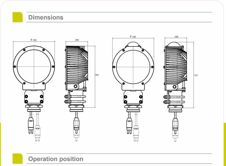
The Elevated 797 fixture is for outdoor use only. The operation position must be according the drawing (note: drawing is indicative only).
