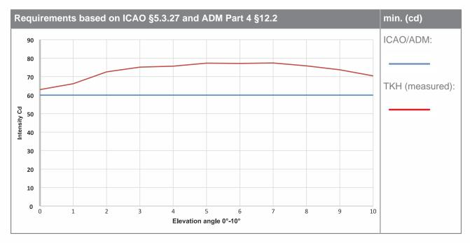
This candela diagram shows a single section of the full 360° diagram.
