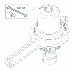
Carefully release and remove the 2 parts of the HIRE assembly tool.
