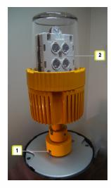
**12.** Mount the CEDD® Elevated Base onto the shallow base with 2 bolts and washers. Tighten the bolts using a calibrated torque wrench to the torque value given in the shallow base installation instructions.
