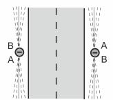
**NOTICE** An arrow on the LED module points in the direction of the runway side.
