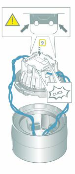
**NOTICE** Do not apply excessive force on the inductive clamp lid, as this could damage the Elevated Base and ferrite parts.
