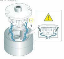
It is important to position the CEDD® Elevated Base in the shallow base correctly to ensure the required light output direction. The positioning screw on the coupling collar (1) must be aligned opposite to the runway arrow (2) on the LED module in the fixture.
