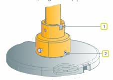
**4.** Press the fixture down firmly until the connector plugs into the receptacle on top of the CEDD<sup>®</sup> Elevated Base.
