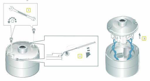
2. Pry the CEDD® Elevated Base out of the shallow base using the lifting tool.
