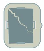
If the I-plate is damaged (chipped or broken) it needs to be replaced. Contact TKH Airport Solutions Customer Service.
