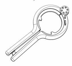
HIRE Adjustment Tool 796101 (see *Aligning the Lights* on page 20)
