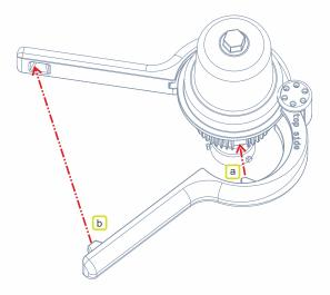
10 Hold the handles of the holder key and use a torque wrench with SW32 nut to tighten the nut on top of the mounting hood to 40 Nm. This will tighten the yellow plastic ring onto the fixture.
