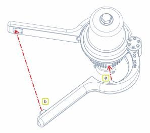
3 Hold the handles of the holder key and use a SW32 wrench to turn the nut on top of the mounting hood by about 30° anticlockwise. This will release the yellow plastic ring.
