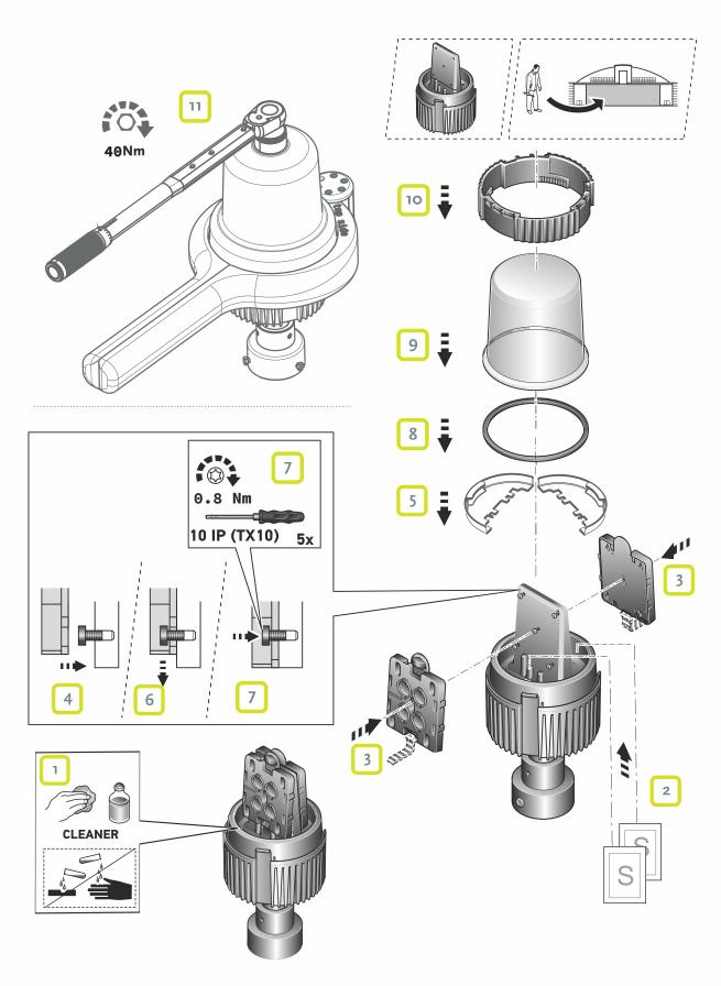
**NOTICE** To close the fixture tightly, use the HIRE Assembly Tool (*Closing the Fixture* on page 32).
